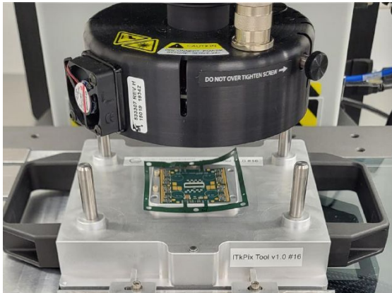
Metrology of silicon pixel modules for the ATLAS inner tracker upgrade (Daniel Perez @ Argonne National Lab)
