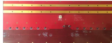
Backplane: Power and signals distribution
