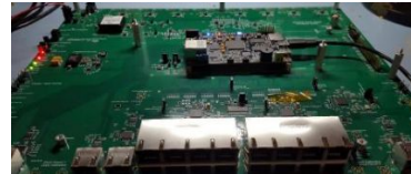
MCB: Clock and beam trigger distribution
