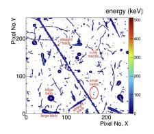
Example of how clustering, ToT and timing can be used to eliminate background and do PID.
