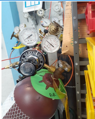
leak test using Ar/iC4H10
