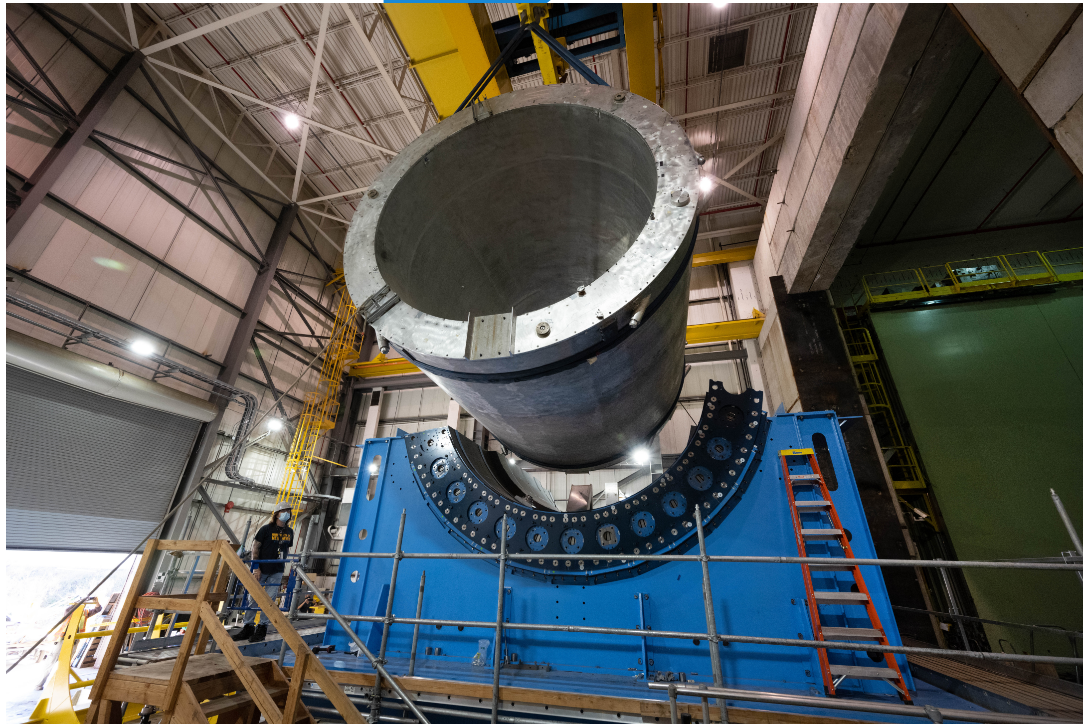
BaBar solenoid installed in sPHENIX IR (October 2021)
