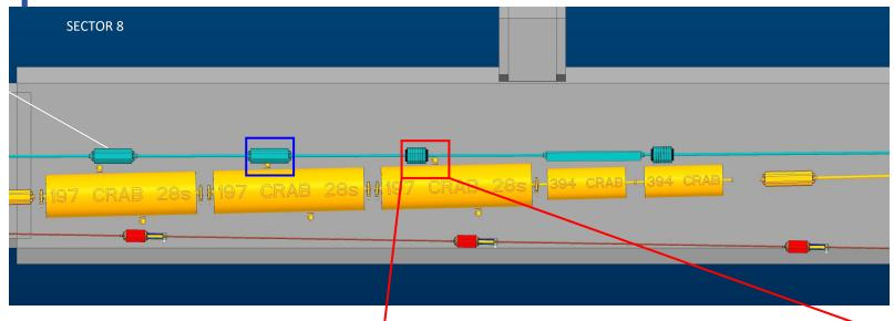
Fixed by moving the IP to x=0.65m from x=0.85 which also helped clearing the forward side hadron crab cavities from the wall.
