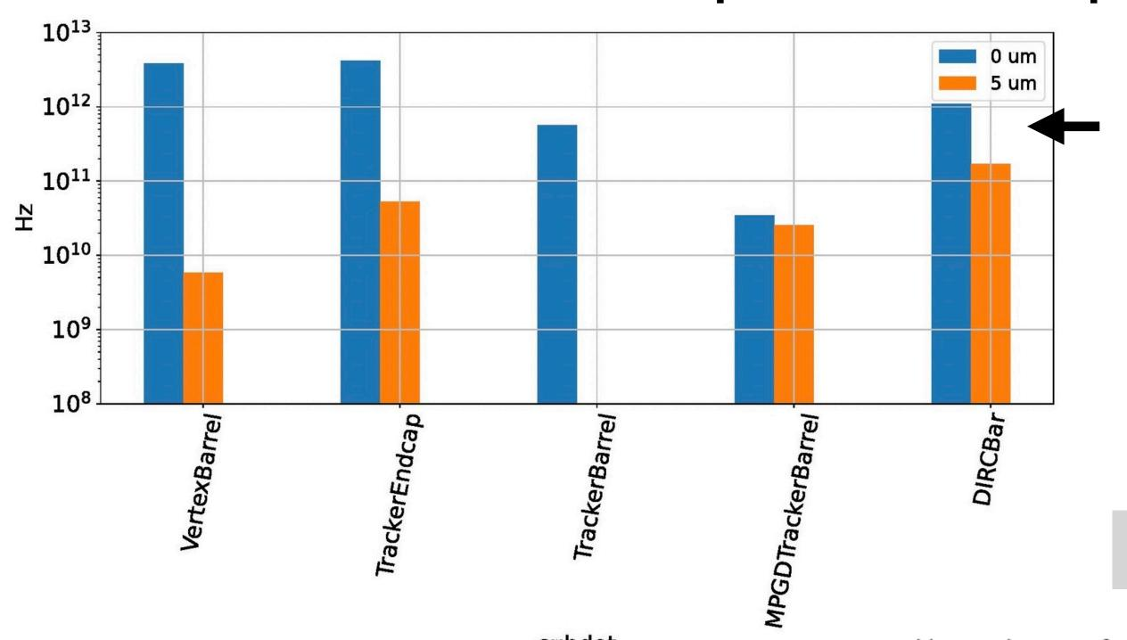
Old (biased) method in which we passed all photons through Geant only once and scaled the resulting contribution by the provided weight.
