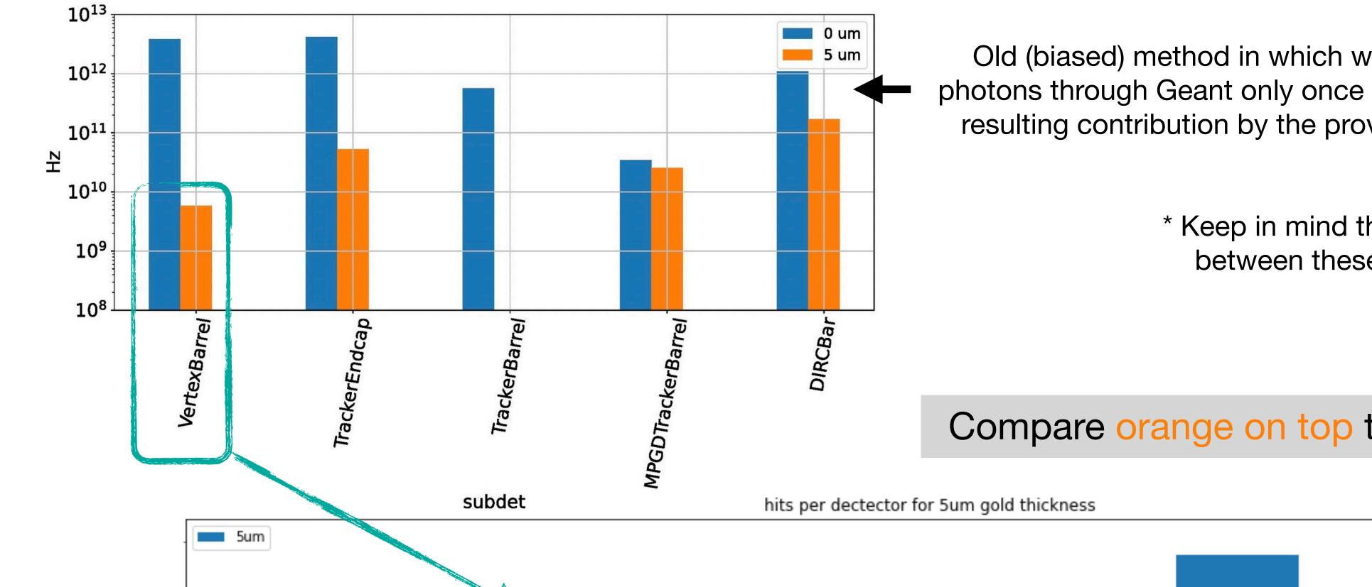
Old (biased) method in which we passed all photons through Geant only once and scaled the resulting contribution by the provided weight.
