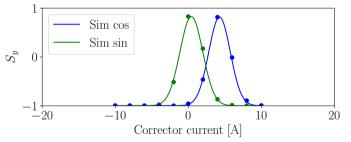
To correct the orbit harmonic h=4,  $[I_{4,S}, I_{4,C}]$ =[2.797 A, 0.669 A] and to spin-flip: h=5 currents are  $[I_{5,S}, I_{5,C}]$ =[10.0 A, -18.0 A] and  $I_{max}$ =23.086 A.
