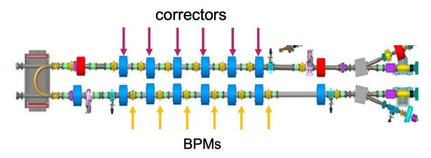
The <u>Goal</u> is to use BO to tune electron trajectories to maximize the ion cooling rate.
