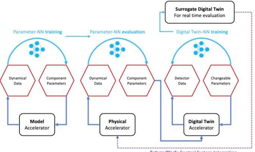
Schematic of how the accelerator model, physical accelerator, and DT of the accelerator are related. The Parameter-NN is trained on the model accelerator dynamical data. This NN is then used to map the dynamic data of the physical accelerator to component parameters of the DT. A separate NN is trained on the output data of the DT, acting as a quick-to-evaluate surrogate of the DT. This Digital-Twin NN maps simulated component parameters to physical accelerator parameters.
