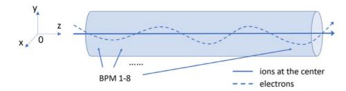
electrons travel through the cooling sections and are monitored by 8 BPMs
