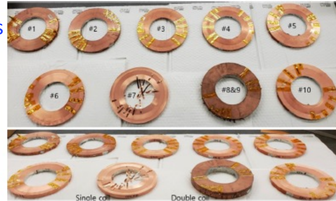
Figure 2.67: Manufacturing process (10 HTS coils). 63
