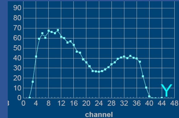
HZB ion beams – two species due to incomplete stripping in tandem
