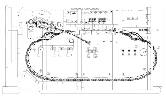
Schematic of the CBETA enclosure. MLC ~10 m for scale.
