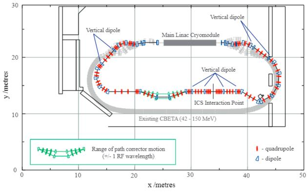
Floor plan schematic of the ICS bypass to CBETA. The existing CBETA return loop is shown in grey. The configurations of the path length correction system are shown in green. Vertical dipoles are indicated.
