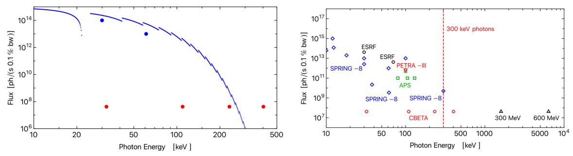
Left: Flux per 0.1% BW of the CBETA ICS (red) against the harmonic curves and data (blue) of the Spring-8 high energy undulator. Right: Flux per 0.1% BW of the CBETA ICS (red) against a collection of the major high energy storage ring undulators across the globe.
