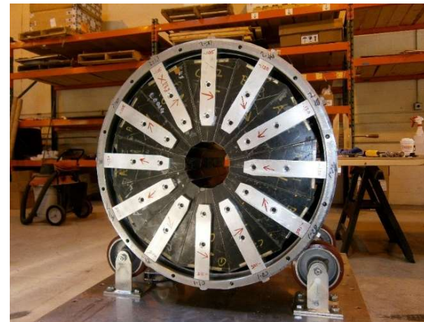
MRI – 1.4 Telsa \text{Ø}110mm \times 400mm 600 kg Nd-B-Fe
