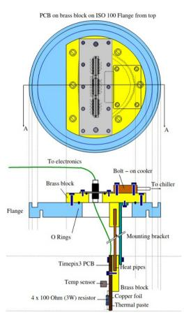
Real **connectors**, vacuum **feedthroughs**, **heat pipes**PCB with **temp sensors**. **Resistors** to mock up ASIC heat.
