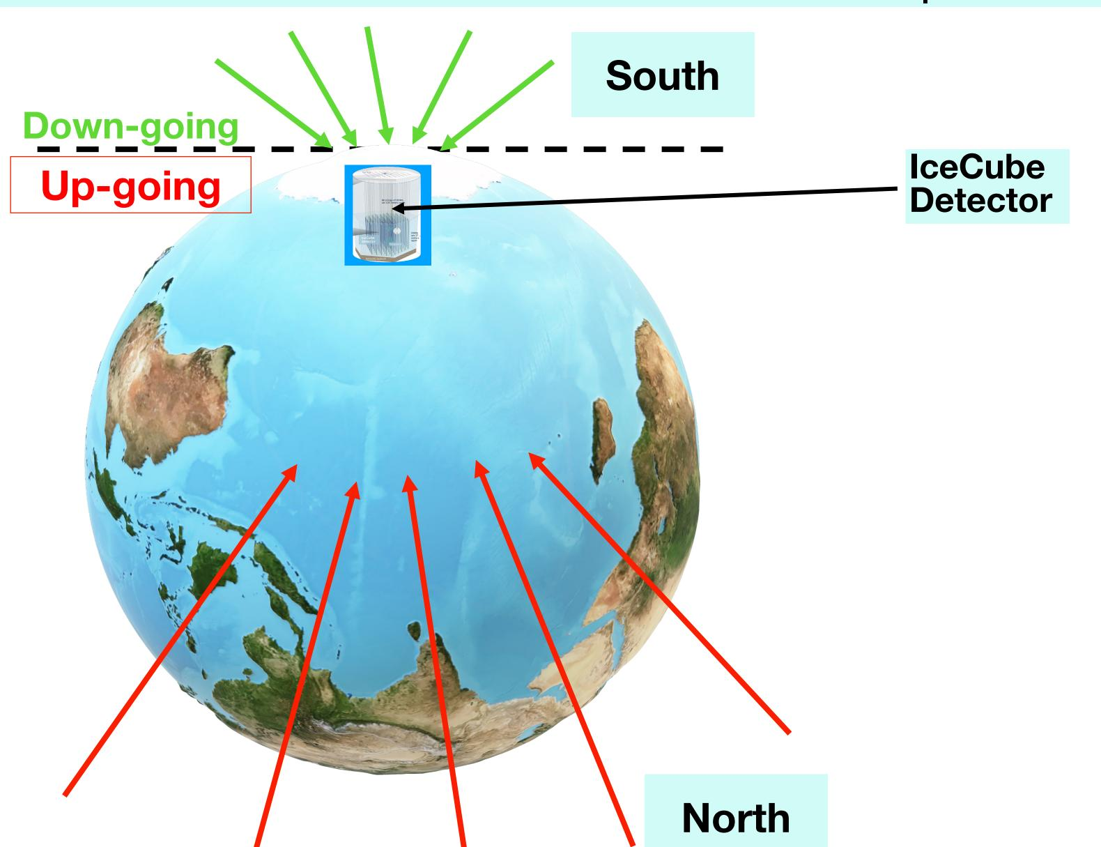
With the increase of neutrino energy, the cross section increases. The up-going events get absorbed by the Earth.
