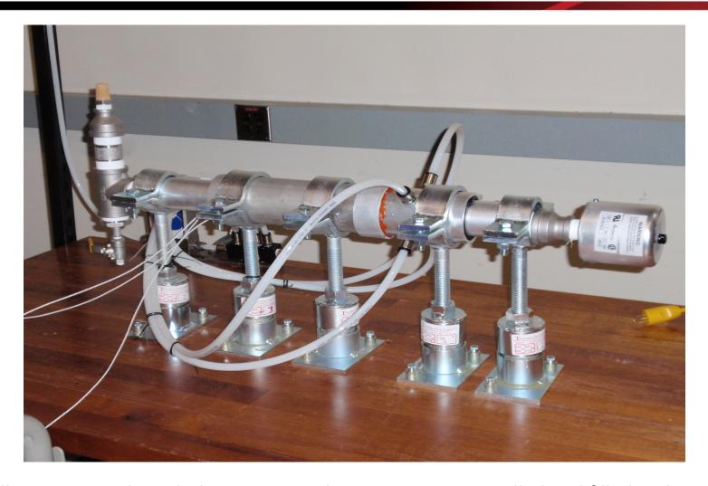
After all pipes were aligned, the immersion heater pipe was installed and filled with mineral oil
