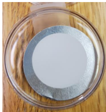
Ba electrodeposition on Al substrate
