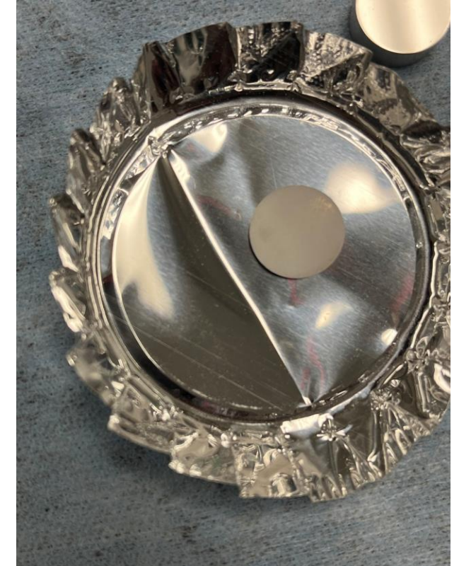
Pressed \text{Ba}(\text{NO}_3)_2 + KBr pellet
