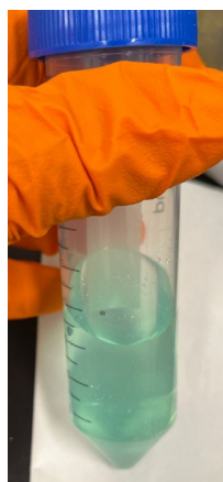
\text{NiSO}_4 \cdot \text{XH}_2\text{O} (462 mg) + (\text{NH}_4)_2\text{SO}_4 (300mg) in water
