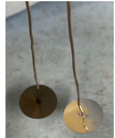
Ni sediments settled on the Pt Anode
