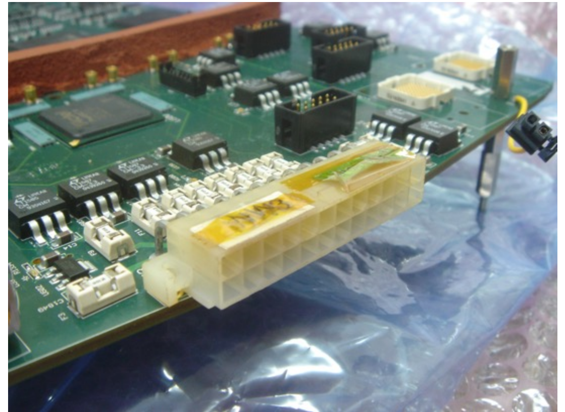
J3 connector was somewhat deformed by the heat
