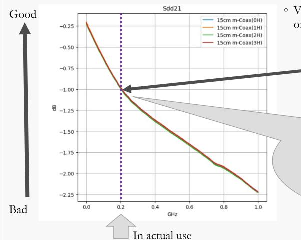
Vertical axis: dB = 20LOG10(S) / Horizontal axis: Frequency of input signal
