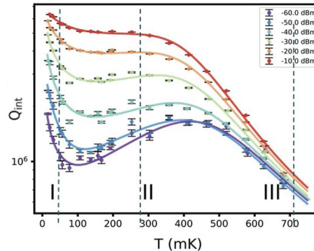
Measuring the Q of tantalum resonators as a function of temperature (x-axis) and power (color lines). Data was fit to a model of two-level system defects in nearby dielectrics. Higher Q indicates lower losses, which means longer photon memory or coherence time.
