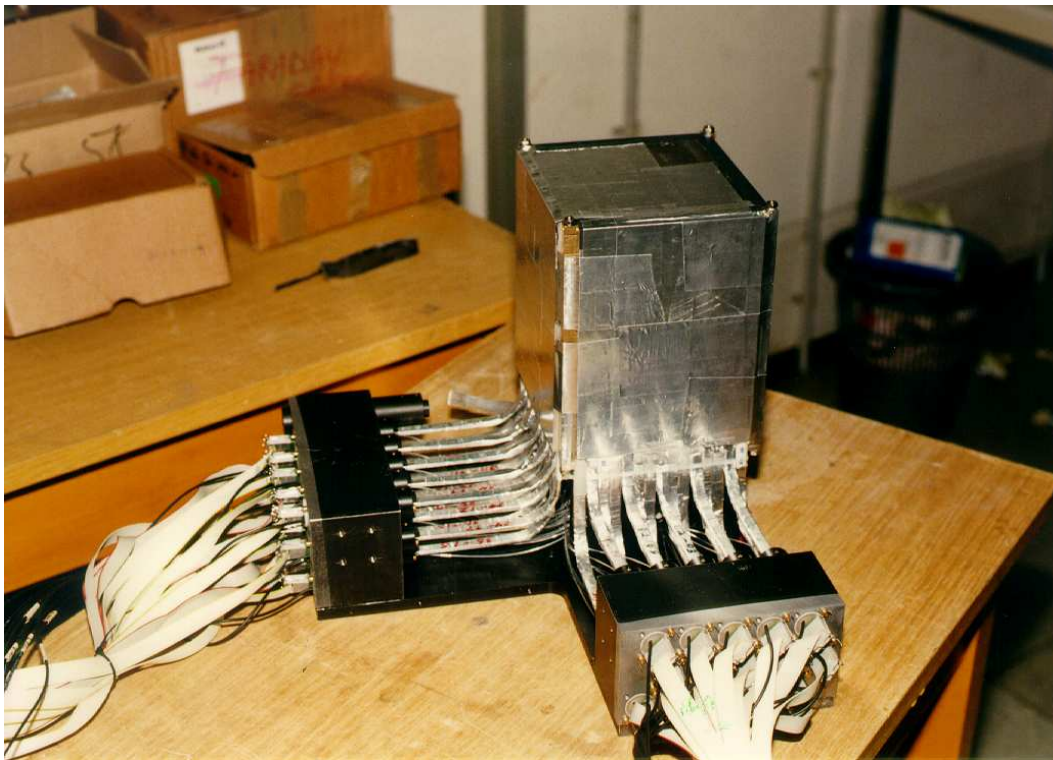
Figure 3.5: The completed, wrapped BPC north module.
