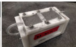
Mold with W powder, fibers + epoxy
