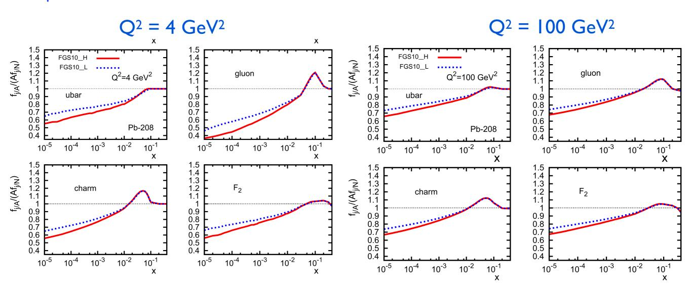
Predictions for nuclear shadowing at the input scale  $Q^2 = 4 \text{ GeV}^2$ . and  $= 100 \text{ GeV}^2$ . The ratios  $R_j$  (u and c quarks and gluons) and  $R_{F2}$  as functions of Bjorken x. Two sets of curves correspond to models FGS10\_H and FGS10\_L.
