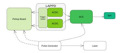
Pulse generator drives laser, sends beamgate to ACC, and in externally-triggered mode, sends trigger signals to the pickup board.
