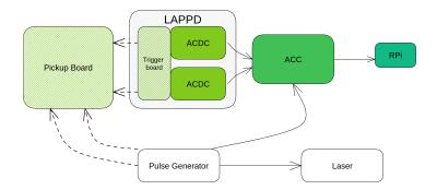
Schematic of the data flow in the dark room setup; dotted arrows are configuration-dependant.
