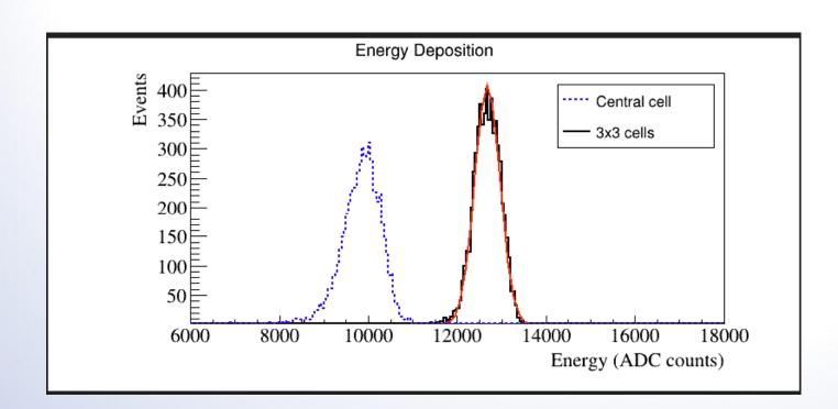
Energy deposition in the central module 5 and in the full prototype (3x3). The energy is given in units of flash ADC counts.
