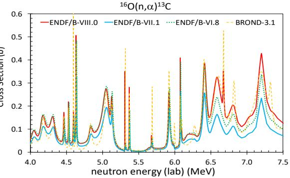
LANSCE measurements (LENZ data), compared with different ENDF releases using the experimental energy resolution function, showed good agreement with ENDF/B-VIII.0 up to 5.5 MeV and ENDF/B-VI above that
