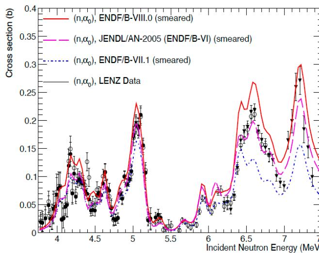
LENZ data: using angular distributions of filled circles - ENDF/B-VIII up to 5.2 MeV
