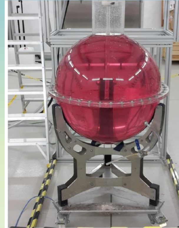
Fig. 1. Photography of manganese bath in lab.
