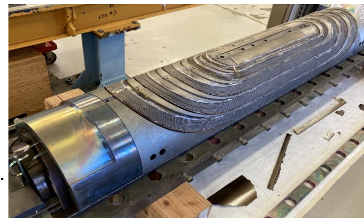
SMCT coil after reaction.
