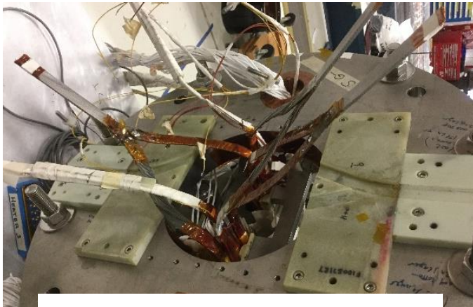
Magnet leads and G10 insulators
