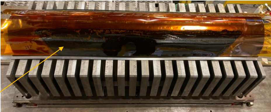
OD casted shim properly located on the coil
