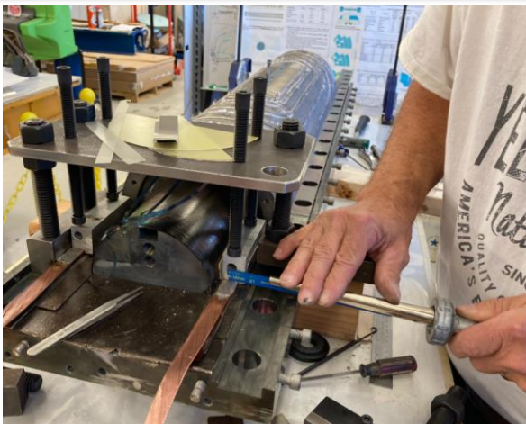
Nb-Ti flexible cables were spliced to Nb 3 Sn coil leads
