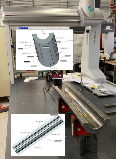
CMM of SMCT impregnated coils
