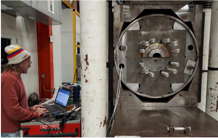
The welding contact tooling in the press
