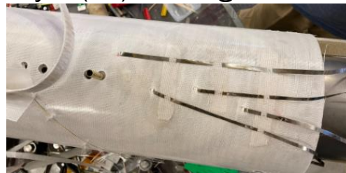
L1 VT strips located between two inter-layer blankets and will be not accessible after HT
