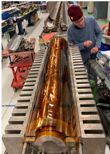
Electrical test before clamping
