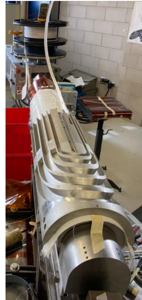
Coil 3D printed mandrel for L2
