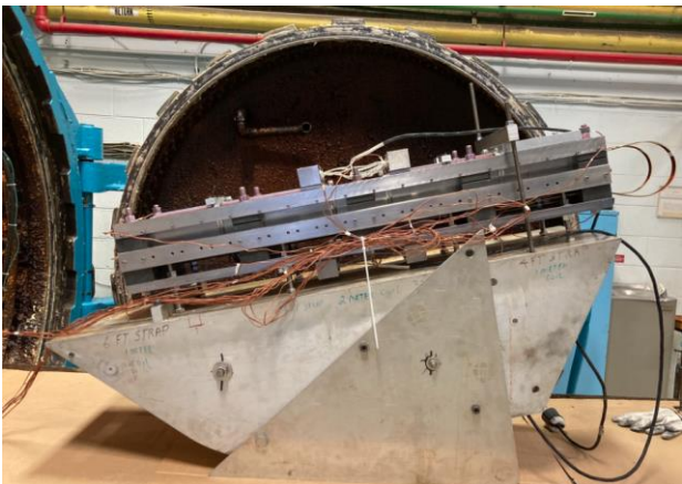
Coil potted with CTD101K epoxy resin, and cured at 125°C for 16 hours
