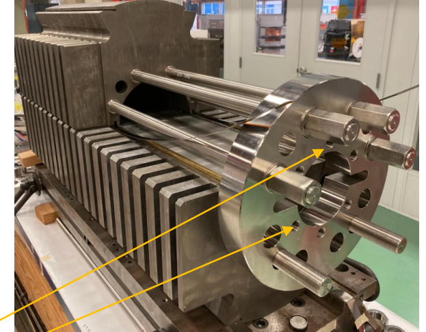
Outer coil support anchoring in the iron middle
