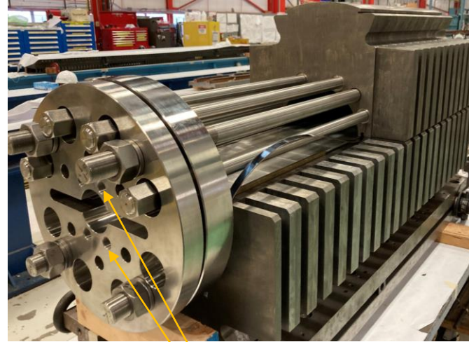
Inner coil support anchored to the iron ends
