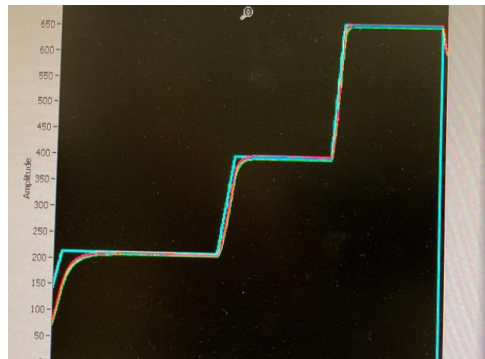
200h 3-step reaction cycle with T_{max}=658^{\circ}\text{C}/48\text{h} in Argon gas
