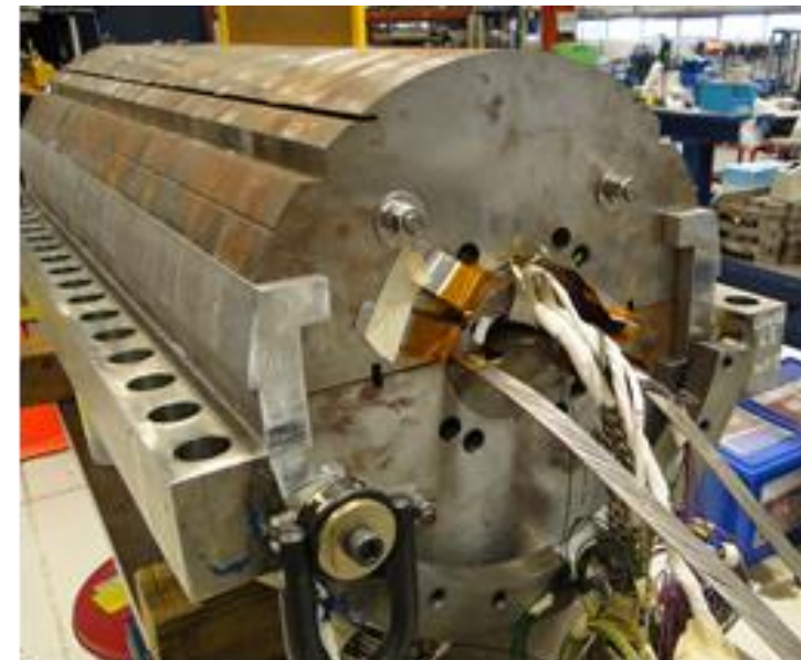
Dipole structure developed at Fermilab and used to test superconducting dipole coils.
