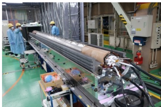
Collared coil on bottom yoke
