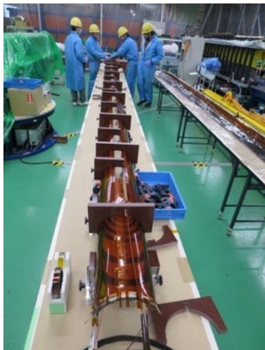
QPH, ground insulation wrapping
