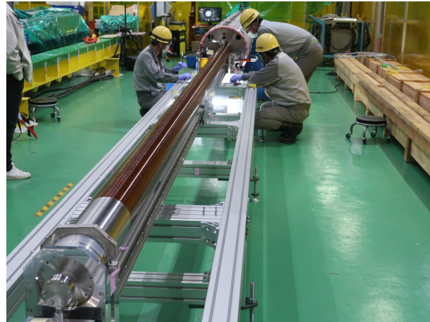
Beam Tube Insertion
