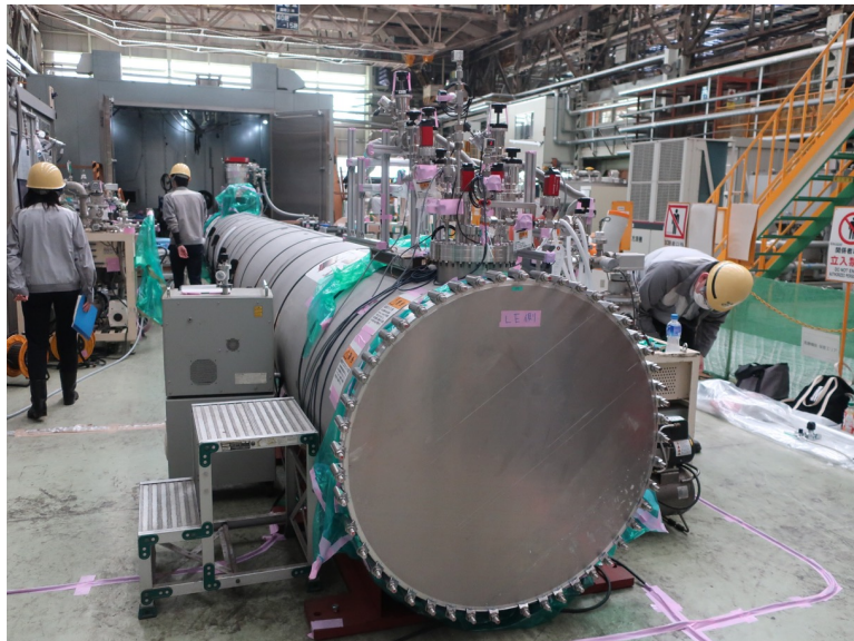
Final Leak Check
