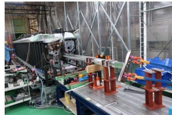
Removal of collaring mandrel
