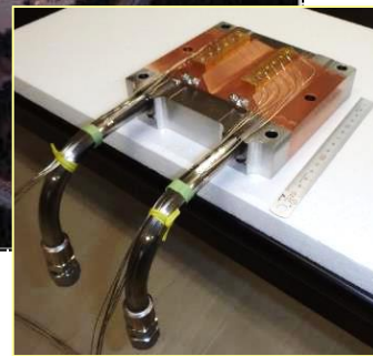
Hadron [HEF] Water cooled gold/ high-Z rotating target
