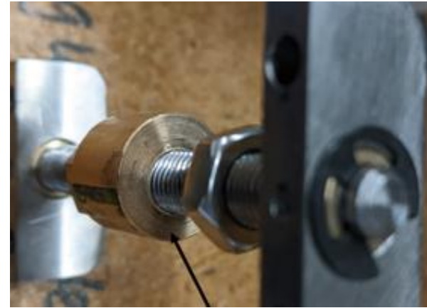
Eccentric top roller accommodate variation in thickness
