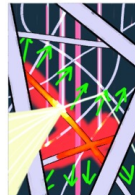
4. Helium around fibers heat, starts convection
