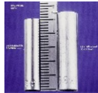
Dimensional change due to void swelling (Porter et al., 1988)
