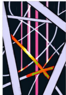
2. Beam hits: fibers instantly heat and conduction starts
