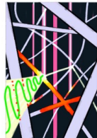
3. Radiation is emitted from hot fibers
