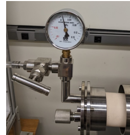
Furnace reconfiguration for heat-treatment of nanofibers in inert gas environment
