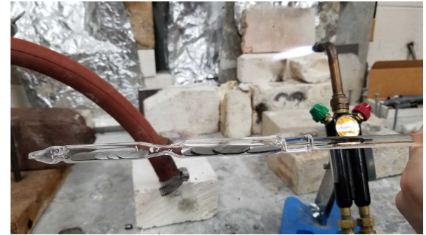
HEA samples sealed in quartz under vacuum before heat treatment (UW-Madison)
