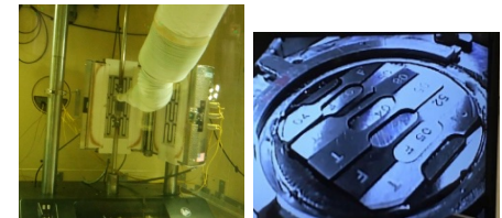
Tensile testing in PNNL hot cells
