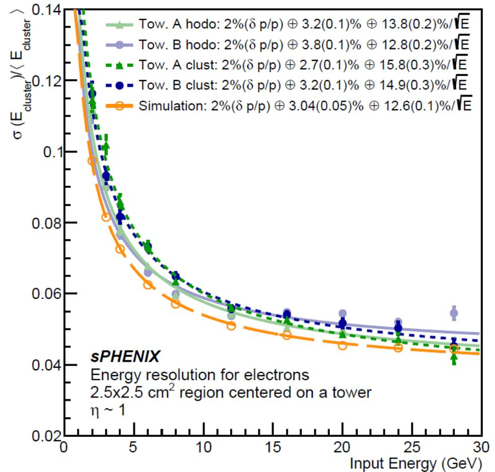
Design and Beam Test Results for the 2D Projective sPHENIX Electromagnetic Calorimeter Prototype (arXiv:2003.13685)
