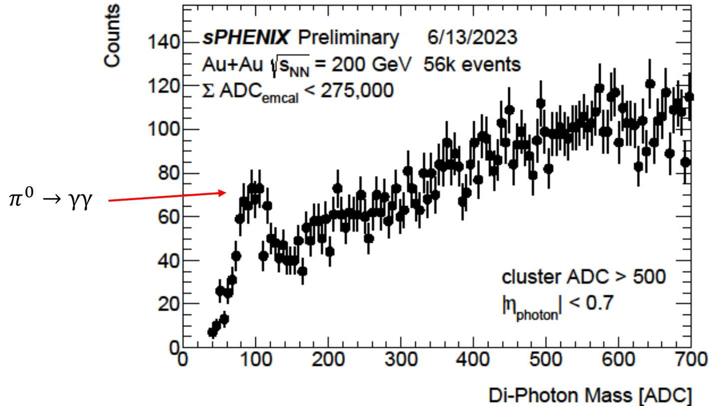
The di-photon mass distribution in units of ADC.  $\pi^0$  peak around 90-100 ADC.
