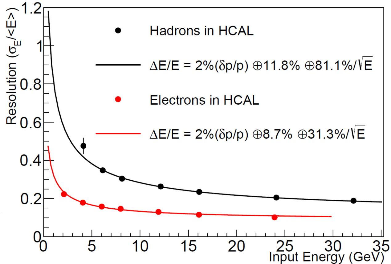
Design and Beam Test Results for the sPHENIX Electromagnetic and Hadronic Calorimeter Prototypes (arXiv:1704.01461)
