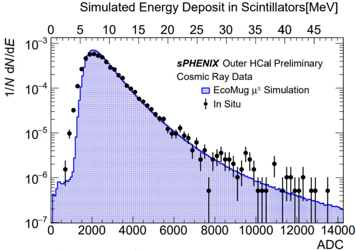
Overall tower's MIP cosmic energy spectrum (with direction perpendicular to radius)
