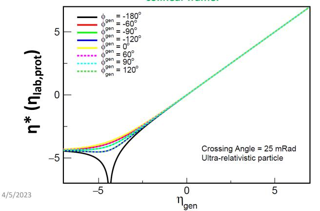
Acceptance cut of, for example,  $\eta^* (\eta_{lab,prot}) < +4.0$  does <u>not</u> lead to a  $\varphi$  dependent acceptance in the colinear frame.
