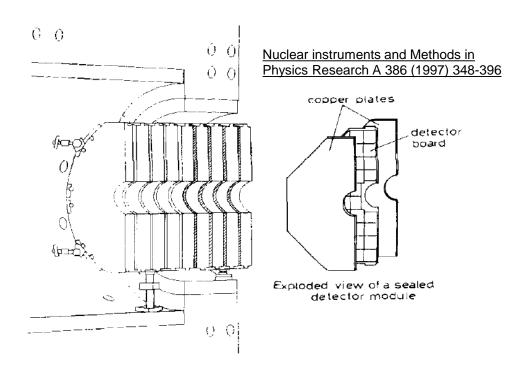
Our motivation for an insert (plug) calorimeter at the EIC is similar. The technology we will use is, of course, quite different. "[The Plug's] main task is to minimise the missing part of the total transverse momentum due to hadrons emitted close to the beam pipe. In addition the energy, emitted into a narrow cone around the beam pipe can be used to separate the proton jet as well as to veto beam gas and beam wall background."
