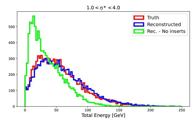
For all events with  $Q^2 > 100 \text{ GeV}^2$ , the red curve shows the true energy of the generated particles in the  $1 < \eta^* < 4$  range. The blue curve shows the reconstructed energy when the
