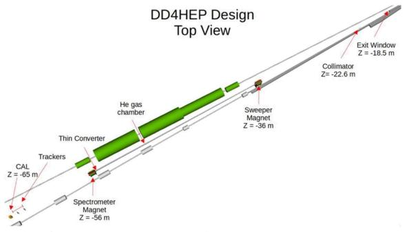
The detector will provide complementary information needed for the precise luminosity determination (1% on absolute and 10<sup>-4</sup> for relative).
