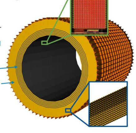
Energy resolution - SciFi/Pb Layers: 5.2%  $\sqrt{E} \oplus 1.0\%$ Position resolution - Imaging Layers (+ 2-side SciFi readout): with 1st layer hit information ~ pixel size for y
