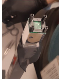
Assembly of SiPM and crystal/glass blocks
