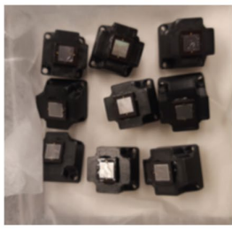
Assembly of SiPM and crystal/glass blocks
