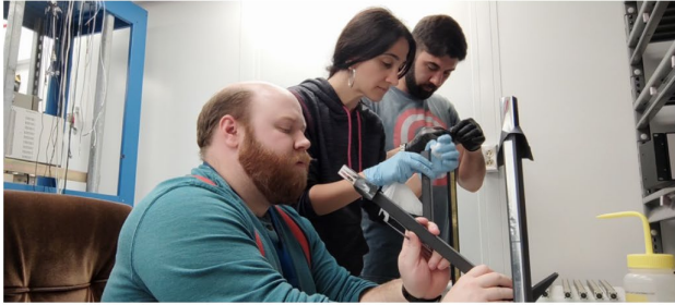
Assembly of SiPM and crystal/glass blocks
