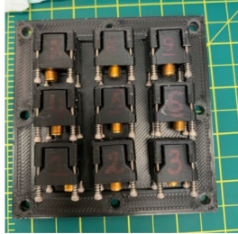
Assembly of SiPM and crystal/glass blocks
