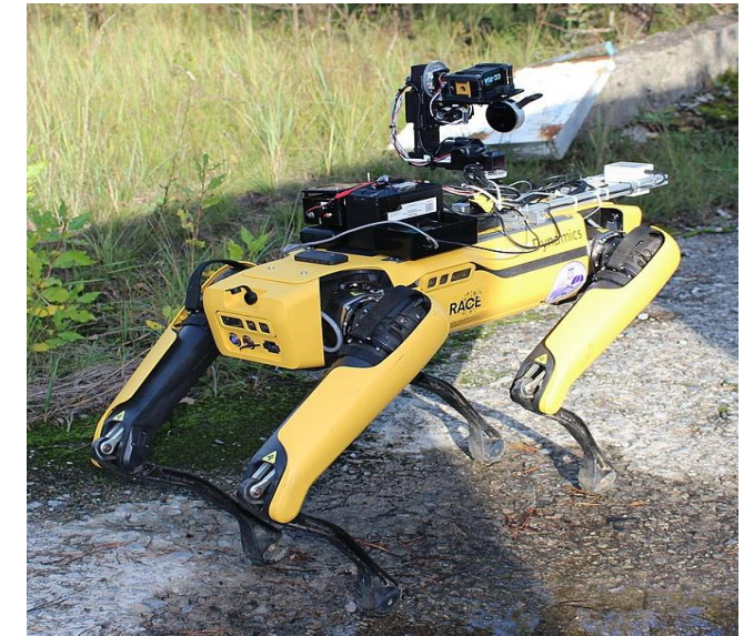
A YanDavos radiation sensor system based on a 1 cm 3 CZT crystal, deployed on a Boston Dynamics Spot quadruped robot for radiation mapping in the Chernobyl Exclusion Zone.
