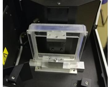
Each tile was placed into a holder (10x10 cm<sup>2</sup>) and mounted onto a metal ridge sliding perpendicular to the beam to explore different positions of the samples
