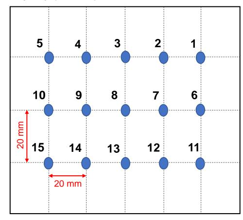
Transmittance measured at 15 different points on the tile
