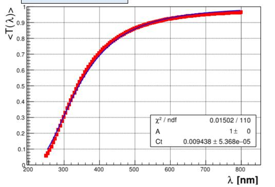
Transmittance fitted by **Hunt extended**:
