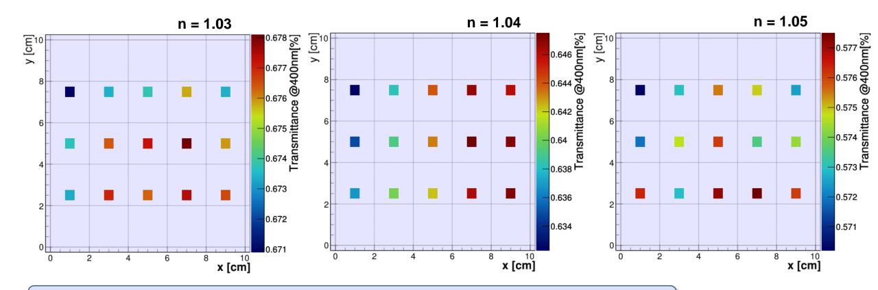
Small transmittance dispersion around 0.6%, which ensures a high uniformity
