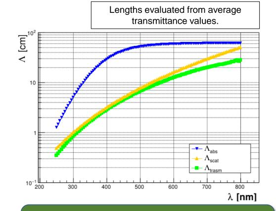
SMALL IMPACT OF THE ABSORPTION ON THE TRANSMISSION LENGTH
