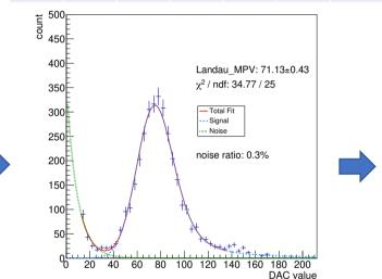
Fitting with Landau+Gaussian convolution function.
