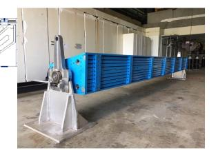
Assembly Detail: 5 scintillators/tower 48 towers per sector 32 sectors; 1536 channels (7680 SiPMs)
