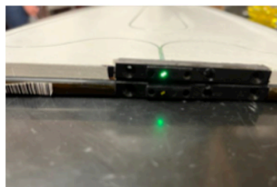
Scintillating Tile exit edge at SiPM location
