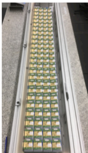
EMCal Sector (96 Towers) with SiPMs and SiPM Daughterboards Mounted
