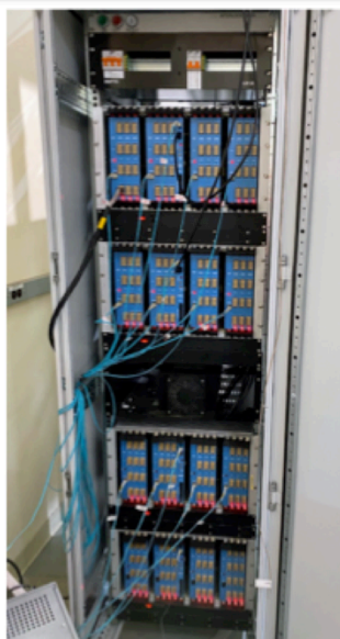
Full Rack of sPHENIX Digitizers assembled and under test
