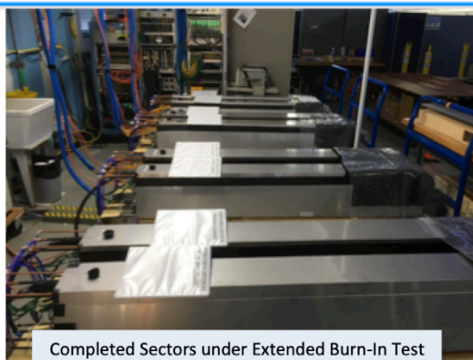
Completed Sectors under Extended Burn-In Test
