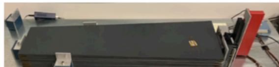
Several Wrapped Scintillating Tiles being checked in the cosmic ray test fixture
