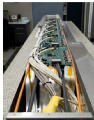
EMCal Sector (96 Towers) with PreAmps, Interface Boards and Cabling Mounted
