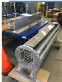
Finished Sectors in the Rotating Test Fixture for Cosmic Tests
