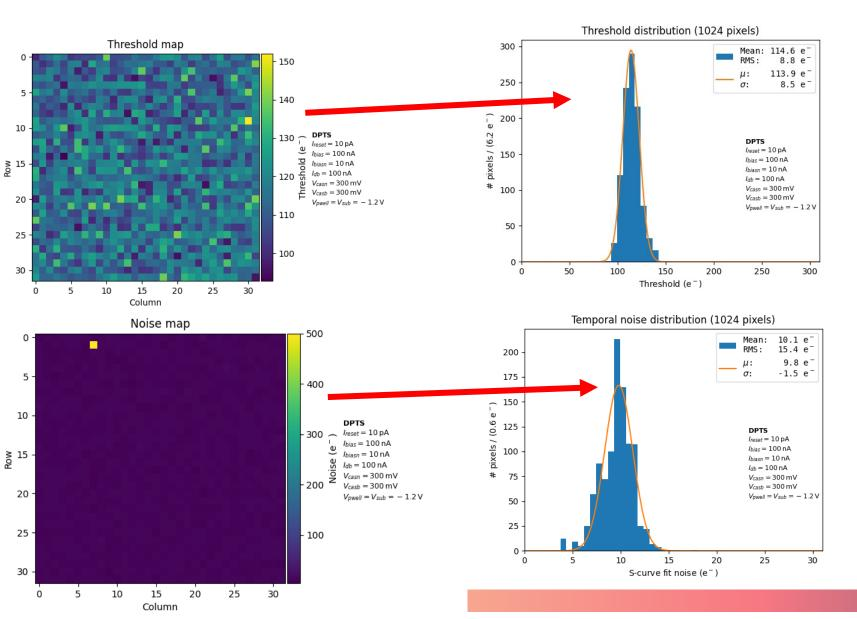
The threshold and noise are determined from the mean and standard deviation of the derivative of the S-Curve.
