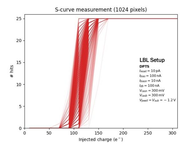
At a given  $V_H$  (i.e. input charge), each pixel is pulsed 25 times and the number of hits is recorded. A hit requires two pulses to be captured by the scope – indicating the assertion and de-assertion of the discriminator pulse.
