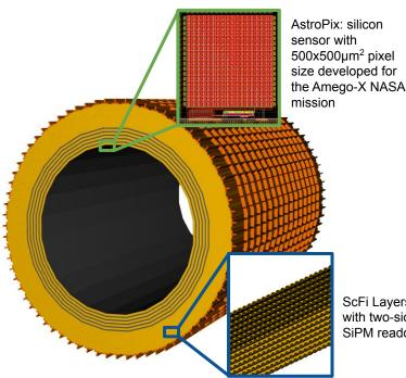
ScFi Layers with two-sided SiPM readout
