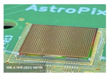
Insert layers of monolithic AstroPix sensors (inexpensive ultra-low-power silicon sensor developed for NASA) in the first half of the calorimeter to capture a 3-D image of the developing shower
