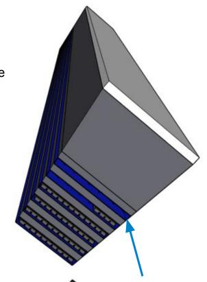
**Shelf** - a carbon fiber structure that is glued to the Pb/ScFi layers, that we will slide trays with AstroPix stayes on.
