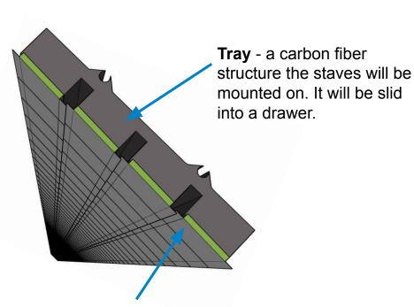
AstroPix **Stave**Consists of 1 x 108 chips with the support structure
