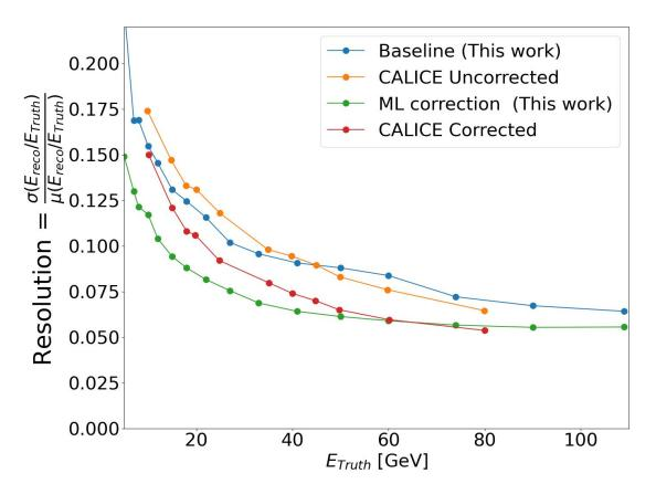
ML based software compensation shows some improvement over traditional software compensation at low energies.
