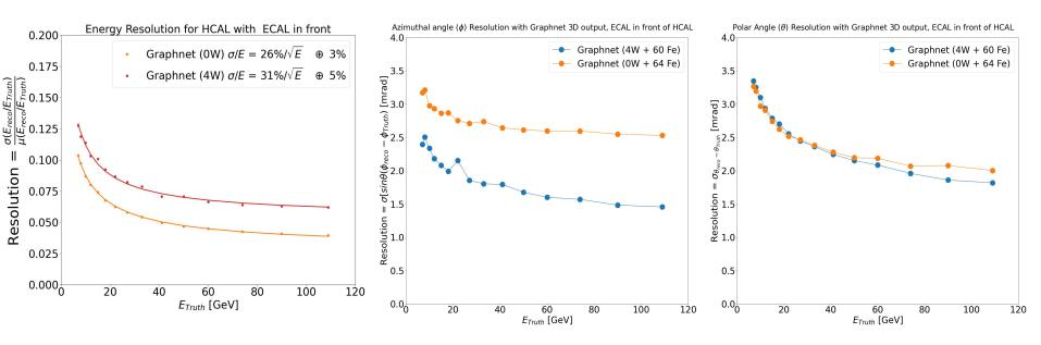
The inclusion of W leads to better azimuthal angle resolution but significantly worse energy resolution. No significant effect on shower containment observed. The overall calorimeter system is deep enough and changes due to W are marginal. ECAL + HCAL (4W + 60Fe), total= $7.7 \lambda$  ECAL + HCAL (0W + 64Fe), total= $7.5 \lambda$
