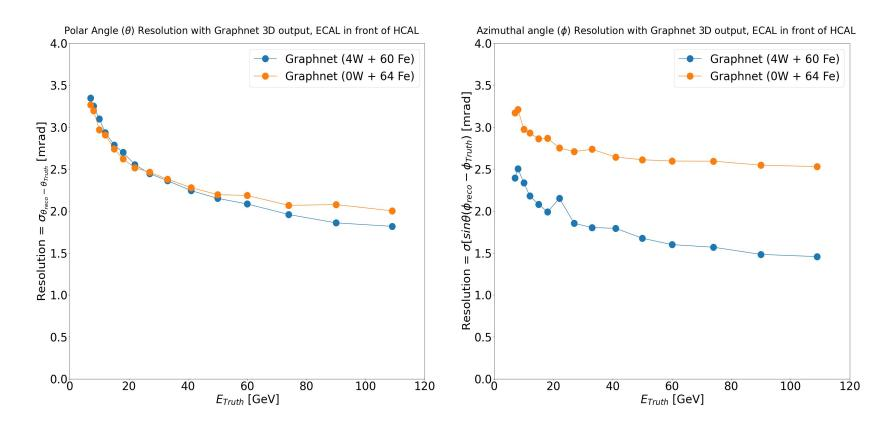
Addition of W layers improves azimuthal angular resolution for azimuthal angle (transverse plane) But not much for polar angle (longitudinal)
