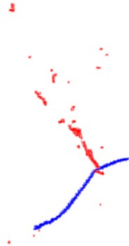
(b) Track/Shower separation
