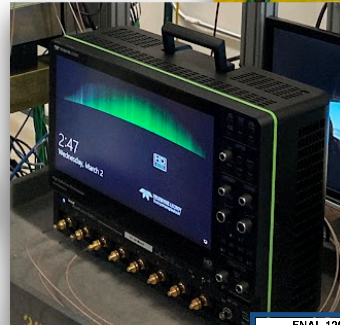
8-channel oscilloscope, 2 GHz, 10 GSa/s
