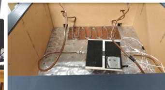
Cold box setup for thermal performance studies of mechanical mock-up modules
